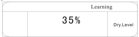
Push "ENT" for the system to learn the level, two beeps will be sounded by the controller, meaning the dry level has been learned. The system returns to the previous menu. The up/down key can be used now to proceed to setting the wet level, or the system will return to normal operation after 20 seconds.
