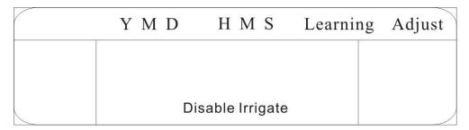
Use the up/down key to cause an icon, which represents an item to set up, to flash, and then select the item by pushing the, "ENT", Enter key into next level menu. Push the exit key, "EXT" to exit. If 20 seconds elapses before a key is pushed the controller will exit from the set up mode, pushing any key while an icon is flashing time will begin a 20 second period to allow data entry again.
